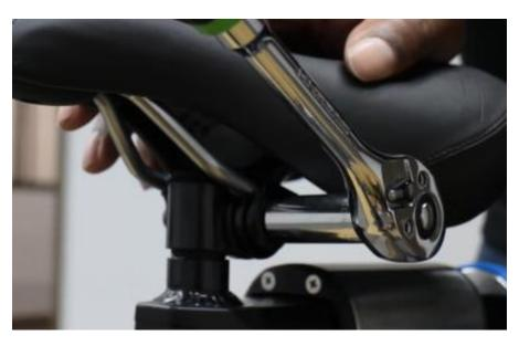
2. Loosen the nuts underneath the new saddle so that the clamp will fit over the seat post (you may need to use a socket wrench).
