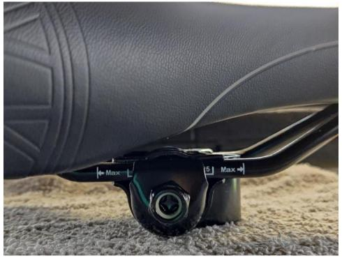
4. Install the new saddle onto the seat post. Tighten each saddle nut **slightly** using a 13mm hex socket - this will make aligning the saddle easier. Once the clamp nuts are tight enough to hold the saddle in place but loose enough to allow you to manipulate the saddle's positioning, align the saddle so that it points straight towards the handlebars and is level with the floor (or to the user's preference).
