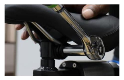
2. Use a 13mm hex to remove one of the clamp nuts, then grasp the remaining nut and pull the shaft out of the clamp. Remove the remaining pieces of the clamp from the saddle and discard.
