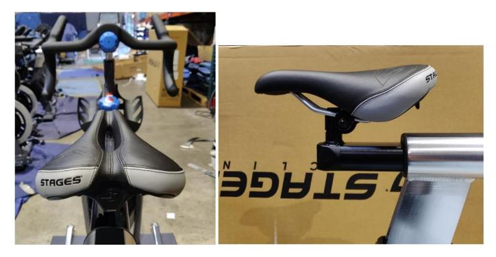
5. Once satisfied with the saddle alignment, use a 13mm hex socket to **FIRMLY** tighten both saddle nuts. Alternate back and forth between each nut so that you tighten them as evenly as possible.
