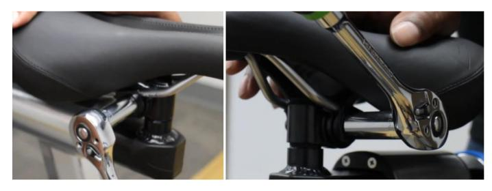
6. Verify that the clamp shaft is not protruding more than slightly through either clamp nut. If the shaft is protruding too far on one side, loosen that side several turns and then tighten the other side to pull the shaft further that direction. Repeat as necessary.
