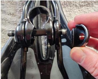
8. Install the nuts back onto both ends of the shaft by hand (only a few threads for now).
