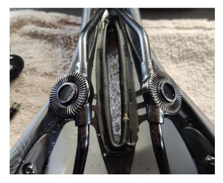
5. The U-shaped center piece of the clamp has complementary grooves that interface with the grooves of the internal clamps. Pivot one of the internal clamps upward **while keeping the saddle rail within the channel** and bring the center piece into contact with it. Rotate the center piece slightly back and forth until you feel the grooves of both surfaces mesh together.
