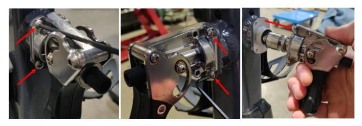
4. Insert the fully assembled pop-pin core into the frame of the bike, then secure it into place using 4 screws and a **hexagonal-tipped** 2.5mm hex.
