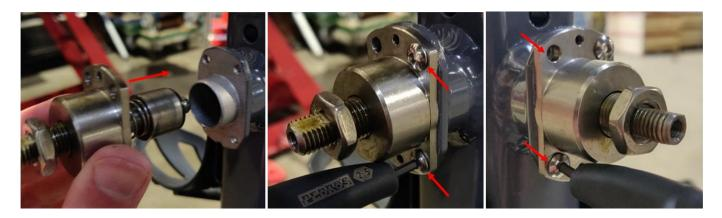
5. Slide the plastic cover over the pop-pin core and use a 2mm hex to secure it in place using 2 screws.
