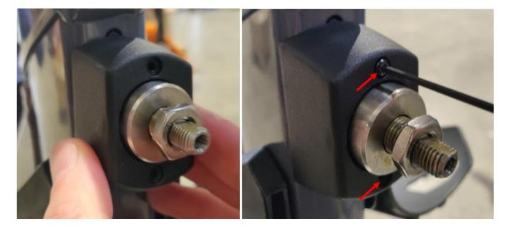
6. The interface of the pop-pin knob and the pop-pin shaft is not round (see red lines in photos below). Align the knob and shaft so that the flat portions match up, then secure the knob to the shaft using a screw, a lock washer, and a 3mm hex.
