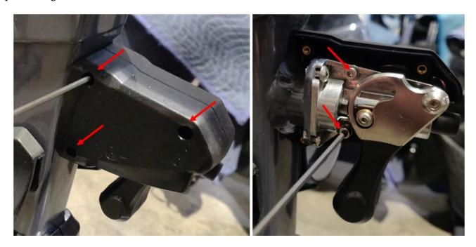
3. Use a **hexagonal-tipped** 2.5mm hex to remove the Fitloc core from the bike frame (2 screws on each side). A long T-handle or the short side of a standard hex key is most effective for removing these screws.
