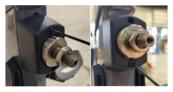
5. **For SC1 models:** Use a crescent/adjustable wrench to break free the larger nut on the pop-pin assembly, then continue to loosen the nut with your fingers until you can remove the assembly from the frame.
