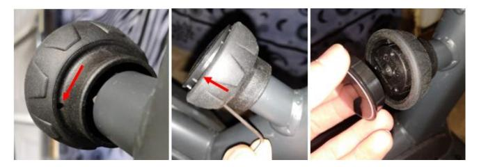
3. Use a 3mm hex to remove the screw from the center of the pop-pin, then remove the pop-pin knob.
