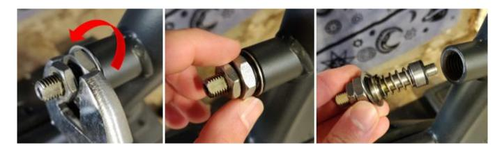
**For all other models:** Use a 2.5mm hex to remove 4 screws from the pop-pin core, then remove the core from the frame.
