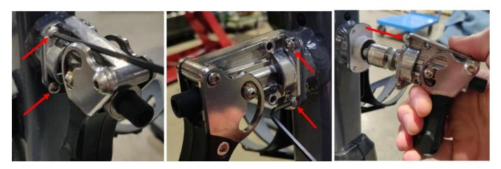
5. Reinstall the Fitloc using the new screws and nuts. When inserting the new core into the frame you may need to pull the seat/handlebar stem slightly upward so that the pin of the Fitloc inserts fully into one of the holes in the stem and sits flush against the frame. See third photo below for side-profile view showing proper nut installation.
