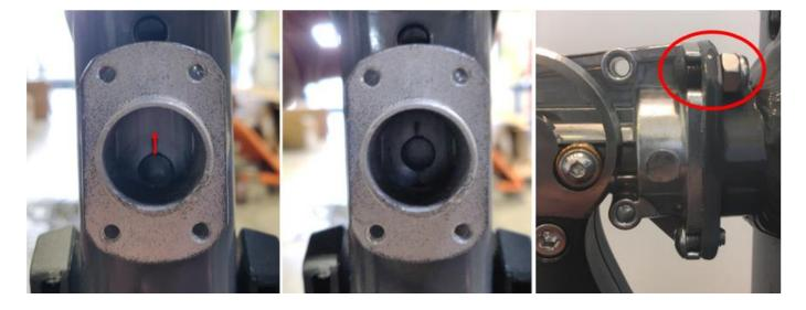
6. Reinstall the Fitloc shroud using a 2.5mm hex (see step 2 for reference photos).
