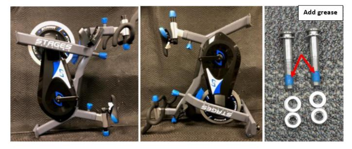
Give the bike another quick test ride. If it is still making noise, the next step is to install gaskets between the stabilizers and the frame of the bike -> Stabilizer Gasket Installation
