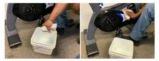
2. Wipe the entire bike clean excluding the seat and handlebar adjustment slides (up/down & fore/aft). It is unnecessary to wash those components unless they are visibly grimy. If you need to clean the adjustment slides, wipe them clean in the same fashion as the rest of the bike, then always be sure to <u>lubricate them</u> afterward using 100% silicone spray.
