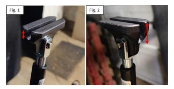
15. To reinstall the handlebar/tablet arm assembly, pull the coiled wire from the bottom of the handlebar stem as taut as you can (Fig. 1) and then thread the wire into the gap in the rear of the list assist head as you bring the handlebar stem down over the head of the lift assist. **Keep the wire as taut as you can.**
