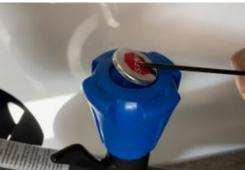
2. Push the knob down firmly and hold it steady with one hand while using a #2 Phillips screwdriver to remove the uncovered screw, then remove the knob itself from the resistance shaft.
