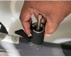
**For stainless steel SprintShifts:** ensure that there is a bushing on the top and bottom of the SprintShift (bushings may be gray plastic or brass).
