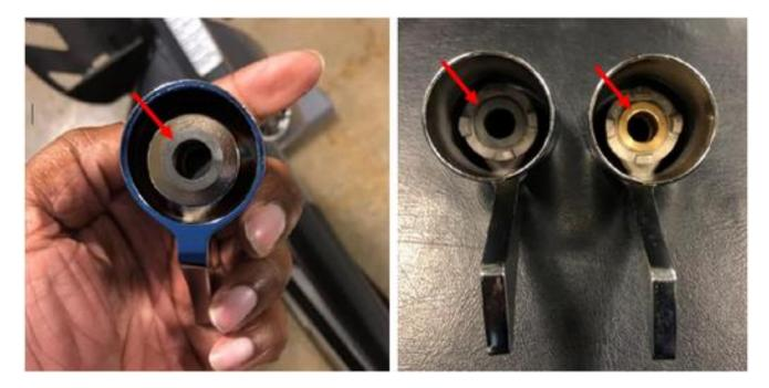
Install the new SprintShift onto the shaft, then the detent, then the spring.
