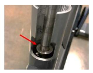
5. **For black plastic SprintShifts:** install the new bottom detent with the protrusion pointing forward, then install the new SprintShift assembly (with the lever pointing straight forward) including the top detent and spring.
