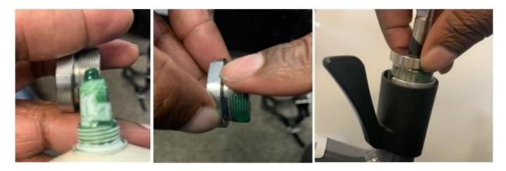
7. Use a medium/large adjustable wrench to finish tightening the cap nut **just until it is snug**.
