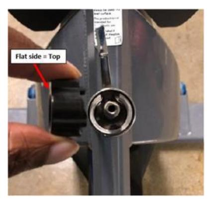
6. Apply a dab of medium thickness grease to the threads of the cap nut and spread it with your finger. Then begin to reinstall the cap nut, threading it as far as you can with your fingers only.
