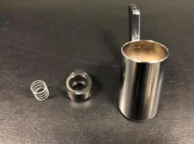
Ensure that there is a metal washer near the bottom of the shaft prior to installing the new SprintShift assembly.
