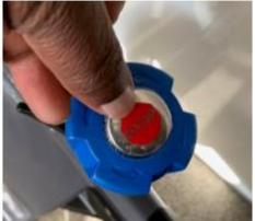
12. Peel the transparent film off the top of the new stop cap.
