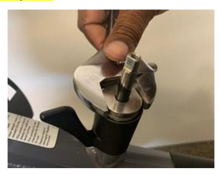
8. Reinstall the resistance knob onto the brake shaft.
