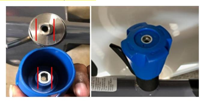
9. Apply a small dab of blue Loctite® onto the resistance knob screw, then reinstall the screw and fully tighten using a #2 screwdriver (again, firmly press the knob down with one hand as you tighten to avoid stripping the screw).
