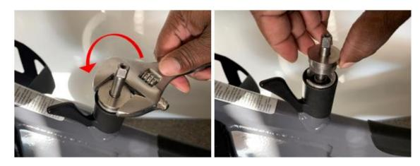
4. **For black plastic SprintShifts:** place the SprintShift lever into the center position (pointing straight forward) and remove it as well as the spring and first plastic detent sitting inside. Then remove the second detent from the brake shaft.
