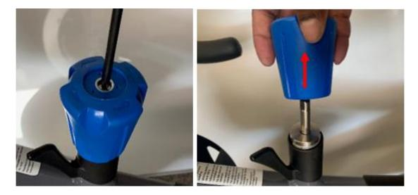
3. Use a medium/large adjustable wrench to break loose the cap nut, then continue to unthread and remove the cap nut with your hand.
