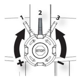
11. Turn the resistance knob counterclockwise until it will not turn any further. Then remove the sticker from the bottom of the new stop cap and install it onto the center of the resistance knob so that it reads **STOP** from left to right.
