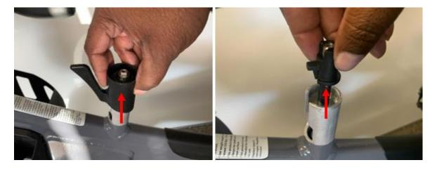
**For stainless steel SprintShifts:** place the SprintShift lever into the center position (pointing straight forward) and then remove it; you can leave the detent and spring inside of the housing.
