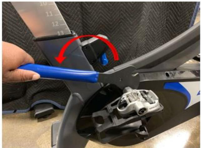
2. Use a size 5mm hex key/socket to remove **four of the five** screws surrounding the user-right crank. Loosen the final screw a few turns but do not fully remove.
