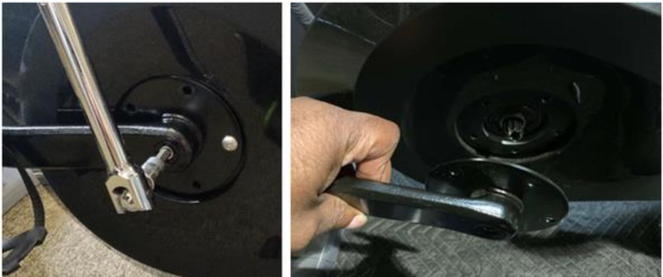
**If the crank bolt is stripped or if the dust cap surrounding the bolt spins as you attempt to remove the crank arm, you will need to remove the dust cap and remove the crank using a crank puller. For those instructions, complete steps 3a - 3b below before proceeding to step 4.**
