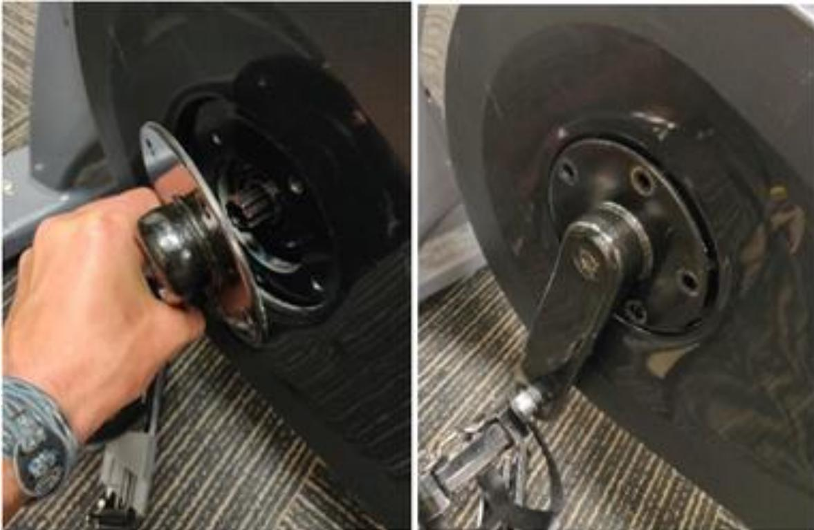
5. Apply blue Loctite to each of the 5mm screws (Fig. 1). Use a small screwdriver or hex key to line up the holes in the crank plate with the drive pulley behind it, then insert the first screw and begin to thread it using a 5mm hex key (do not fully tighten) (Fig. 2). Repeat to insert a second screw (Fig. 3).
