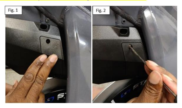
6. Align the screw holes in the nose cone with the screw holes in the frame (one on each side) and secure the nose cone to the frame using the two (2) socket head screws (item **F**) and a 3mm hex key (Fig. 1). Then rotate the water bottle holders on each side back down into place and gently tighten the lower screws using a 2.5mm hex key.
