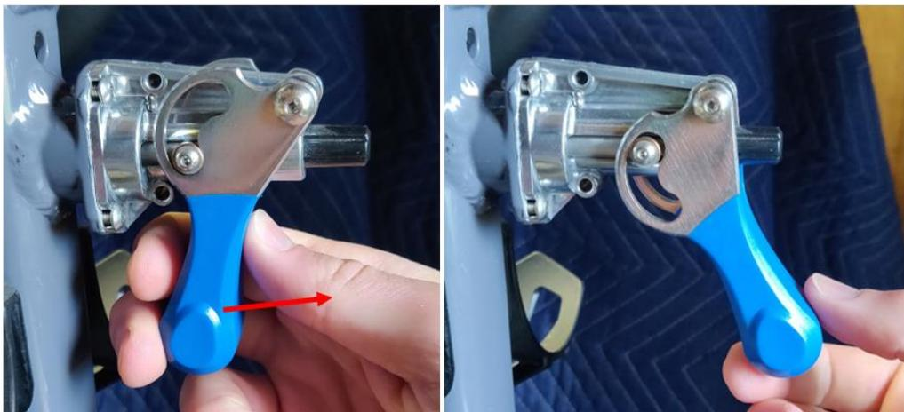
4. Use a 3mm hex and 2mm hex to remove the screws at the top of the Fitloc lever.
