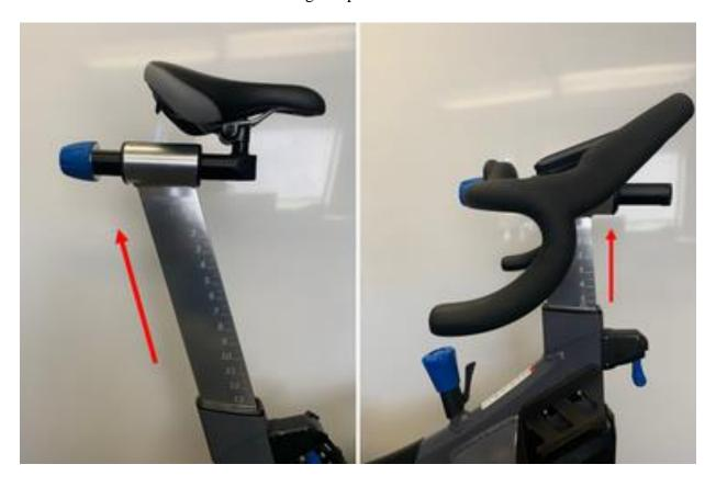
2. Spray the silicone directly onto the seat/handlebar stem while holding the rag/towel behind the stem to catch any errant spray or splash. Repeat on the opposite side of each stem.
