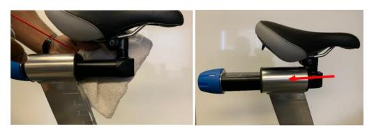
3. Spray some silicone on the rear side of the fore/aft slide, then move the seat/handlebars back and forth a few times to help spread the silicone onto the entire surface.
