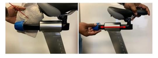
4. Use the rag/towel to spread the silicone around the entire surface of the slide and then wipe off any excess silicone.
