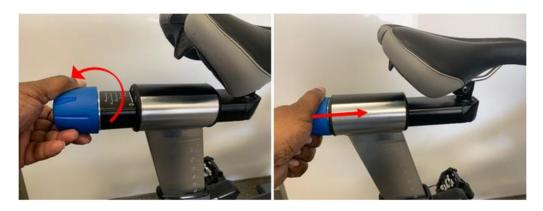
2. Spray some silicone directly onto the exposed surface of the fore/aft slide, then push the seat/handlebars all the way backward.
