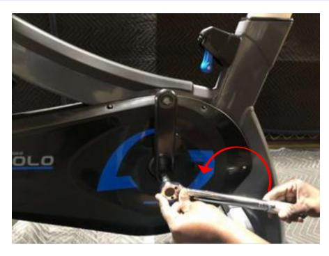
3. Liberally apply some PPL-1 lube (or similar grease) to the exposed splines of the bottom bracket, then attach the new crank arm to the bottom bracket so that it is pointing 180 degrees opposite the right crank.
