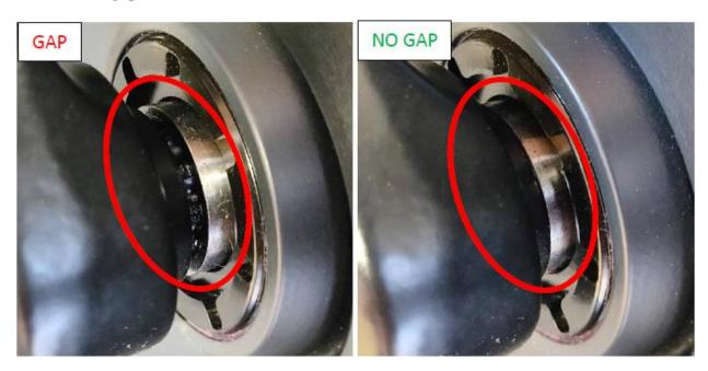
Prior to moving on to the next step, double-check that there is NO GAP between the black of the power meter and the silver of the bottom bracket. If there is a gap, tighten the power meter further (this may require substantial force and/or the use of a breaker bar for added leverage).
