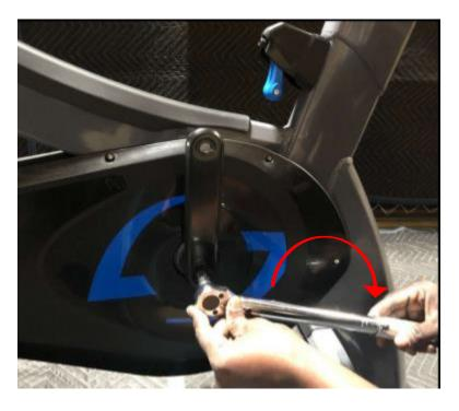
6. Apply a dab of blue LocTite onto the threads of the pedal, then thread it into the crank arm by hand as far as possible (to avoid cross-threading). Finish tightening the pedal very firmly using a 15mm pedal wrench.
