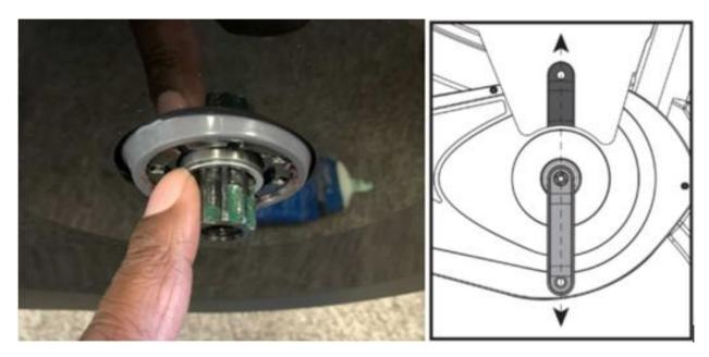
4. Use a socket wrench and 8mm hex bit (ensuring that the tool is fully inserted into the bolt) to tighten the crank arm until it is **BOTTOMED OUT** against the bottom bracket. **There should be no visible gap whatsoever.**
