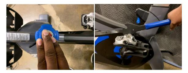
2. Use a socket wrench and 8mm hex socket to remove the crank by way of the embedded self-extracting bolt. Similar to above, holding down the brake with one hand can help to initially break the tension of the bolt free. Be sure that the tool is fully inserted into the bolt before applying any force to help prevent stripping the bolt.
