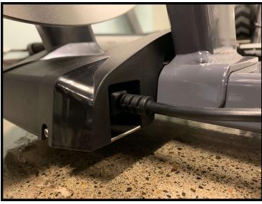
7. Once the new tablet is reinstalled, plug the power cord back into bike.
