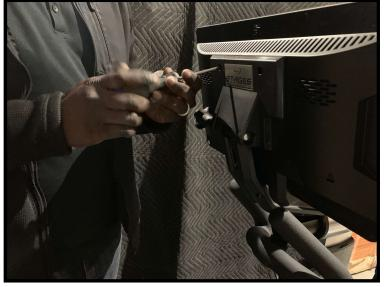
6. Lift up tablet and push the extended power cable back into the tablet bracket (1 to 2 inches pulled out during tablet removal), then reattach the new tablet to the bracket using the four (4) Phillips-head screws.
