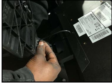
2. Remove the (4) Phillips-head screws from the rear of the tablet. Lay the tablet over and pull out approximately 1 to 2 inches of the power cable from the bracket to give you room to lay the tablet over on top of phone holder.
