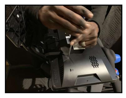
3. Remove the three (3) small screws from the port cover.
