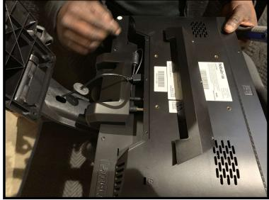
4. Lift and remove port cover from the rear of the tablet.
