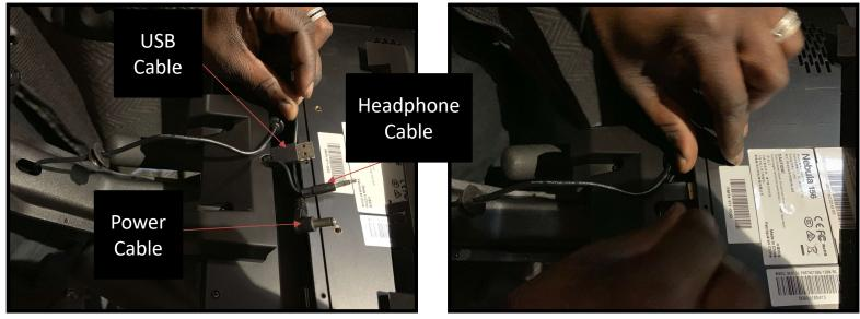
3. Unplug the USB and the headphone cables and then route the power cable from the bike under the USB and headphone cables and plug in. Then, plug in the USB and headphone cables over the power cable on the new tablet.
