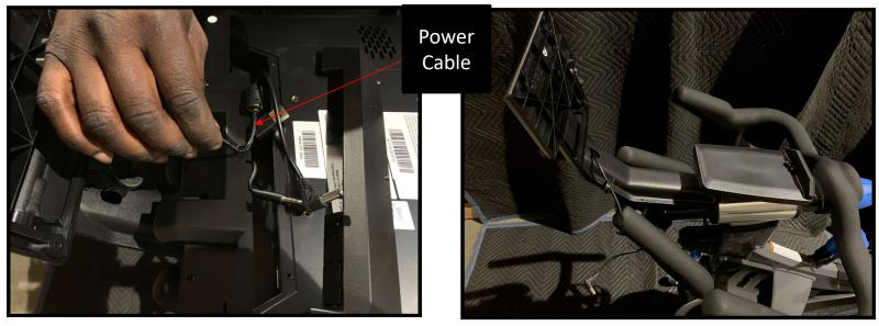
6. Remove the power cable completely from the tablet, then remove the tablet from bike.
