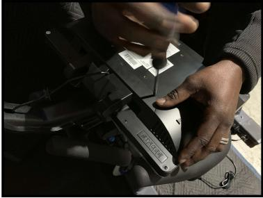
5. Reinstall the port cover onto the tablet with the three (3) small screws and make sure it is flush with the back of the tablet.
