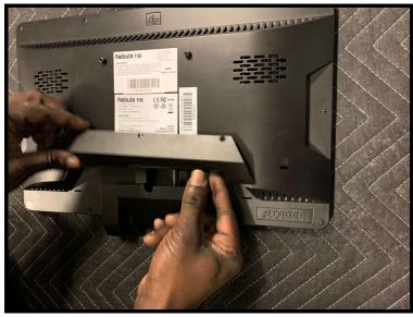
2. Remove the three (3) screws from the port cover and then lift and remove the port cover.
