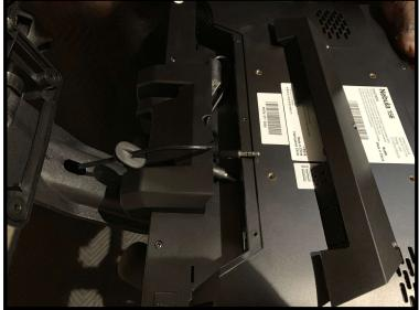
5. Unplug the power cable, USB, and headphone cable from the bottom of the tablet.
