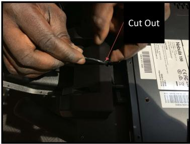
4. Prior to installing port cover, ensure that the in-line filter on the power cable is tucked into the tablet and the power cable is feed through the small cut out on the bottom cover.
